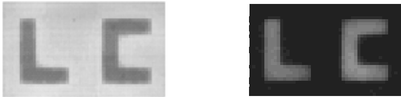
FIGURE 1 Optical images as obtained by Monte Carlo simulations on 50 \times 30 \times 10 lattice. ( Left ): Twisted nematic display, ( Right ): In-plane switching effect display. The applied field strengths are \xi = 1 and \xi = -9 respectively.
