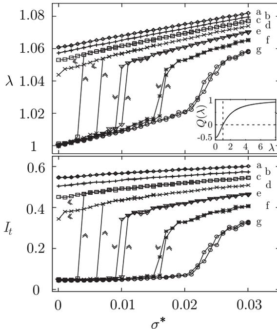
Fig. 2. Regular sample stretched: stress-strain isotherms (*top*) and light transmittance (*bottom*). Curves *a-g* correspond to  $T^* = 1.135 - 1.15$ , with a step size of 0.0025. Arrows denote the scan direction; note the hysteresis. Inset:  $Q(\lambda)$  dependence.
